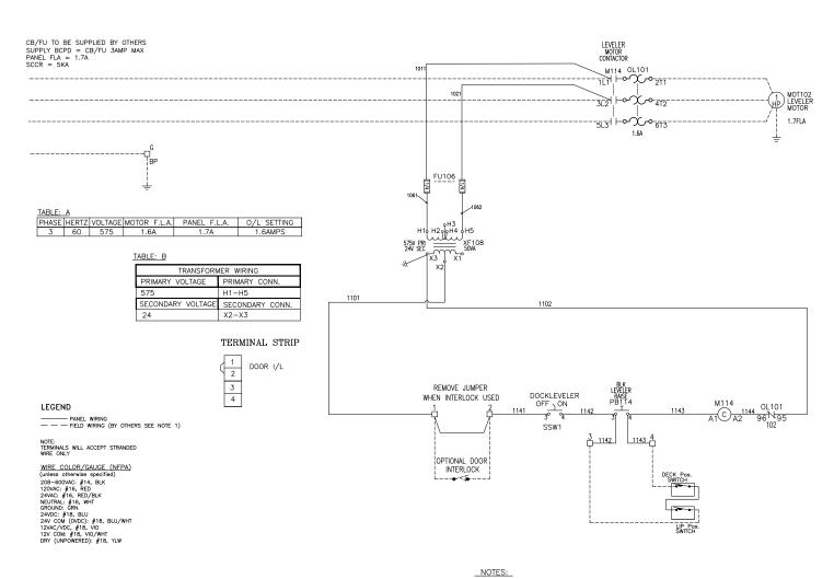
1. FIELD TERMINAL WIRING: 60 / 75 DEGREE WIRE, MIN 16AWG FOR SIGNAL WIRING, MIN 14AWG FOR INCOMING POWER, SEE CHART IN PANEL FOR TORQUE REQUIREMENTS
