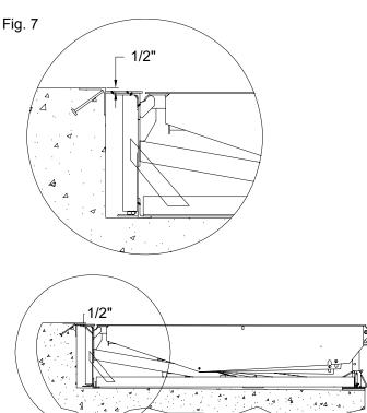
5. Check and adjust the leveler for square and in firm contact with the rear angle. The sides of the leveler should have a 1/2" gap and parallel with the sides of the pit. Tack weld the rear angle to the rear curb angle in 4 places min 3/8" at the center and at both ends. See Fig. 9 and 10.
