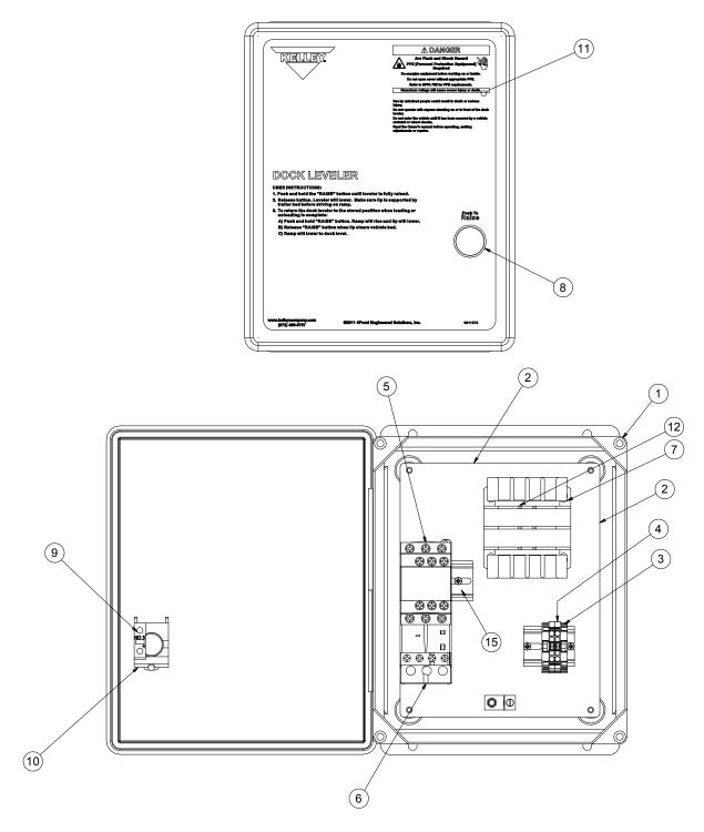
PARTS LIST, continued CONTROL BOX ASSEMBLY WITH OPTIONAL INTERLOCK 6011651 — 575V, 3PH, 60 HZ
