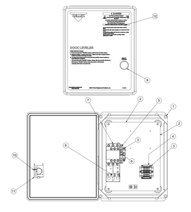
PARTS LIST, continued CONTROL BOX ASSEMBLY WITH OPTIONAL INTERLOCK 6011372 — 120V, 1PH, 60 HZ
