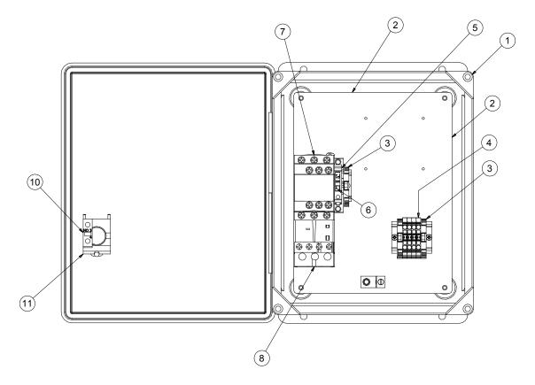
PARTS LIST, continued CONTROL BOX ASSEMBLY WITH OPTIONAL INTERLOCK 6011524 — 208/240V, 1PH, 60 HZ
