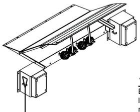
**Top of Dock (TOD) Leveler** This is a version of an EOD leveler and is typically mounted to the floor surface and the leading edge of the dock face of the building. It generally requires minimal or no concrete work. The working range of these units is intended to provide primarily above-dock working range.
