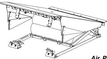
**Air Pit Leveler** This type uses a pneumatic bag system of some type to raise and lower the leveler deck. Obviously, this leveler requires some type of electrical power source - either at the dock or adjacent to it. Most typically, this power source would be standard 110v power. Generally, these levelers are moderately more expensive than mechanical levelers but can involve reduced service and maintenance requirements when compared to mechanical units.
