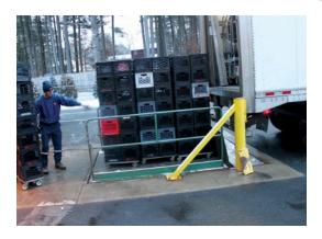
beveled toe guards, a maintenance safety strut, safety chains across the operating ends, upper travel limit switch and a safety tread plate steel deck. Velocity fuses on the lift cylinders prevent the lift from free falling in the event of power loss.
