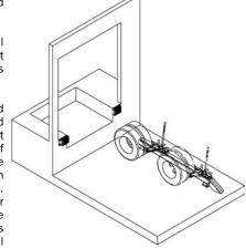
red & green. The operator then pushes the foot pedal, allowing the restraining arm to retract to its stored position. The inside light will remain red and the outside light will turn from red & green flashing to green. It is now safe for the vehicle to leave.
