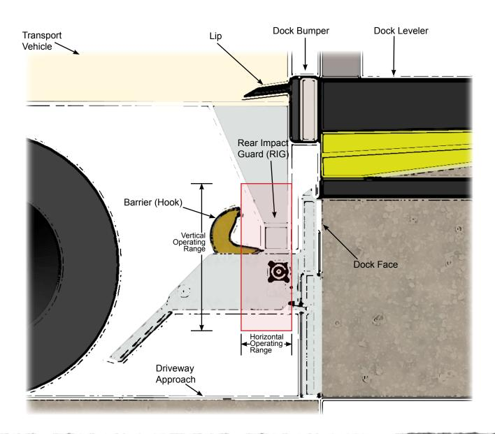
**Automatic Operation:** placement of a vehicle restraint device in its operating position by powered means not initiated by the loading dock operating personnel.
