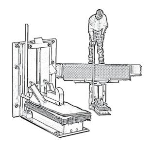
**Power Operated:** A vehicle restraining device that is both engaged and released through a powered means. This is the most popular type of restraint in that the operation is simple and easily accomplished. The restraint is operated by either a simple push button or is automatically engaged as part of an over-all integrated dock system. A light communication package which is part of a powered operated vehicle restraining device is generally sequenced automatically.
