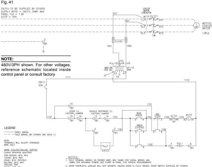
GROUND: GRN 24VDC: #18, BLU 24V COM (0VDC): #18, BLU/WHT 12VAC/VDC, #18, VIO 12V COM: #18, VIO/WHT DRY (UNPOWERED): #18, YLW
