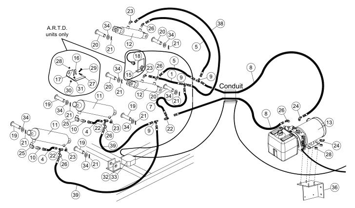
Fig. 50 - Dual Cylinder - 3 Button Control - Remote Mount
