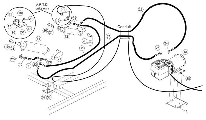
Fig. 47 - Single Cylinder - 3 Button Control - Remote Mount
