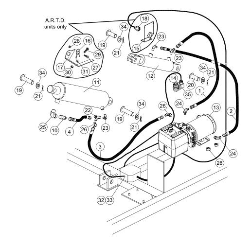
Fig. 46 - Single Cylinder - Single Button Control - Remote Mount
