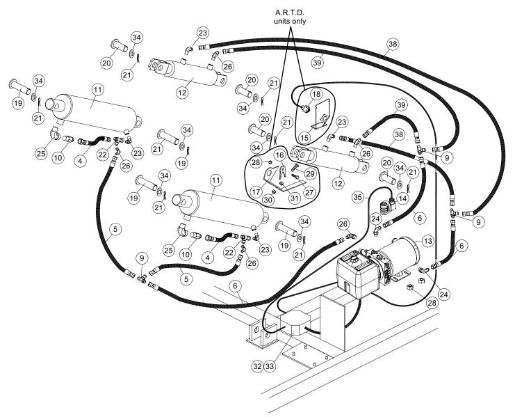
Fig. 49 - Dual Cylinder - Single Button Control - Remote Mount
