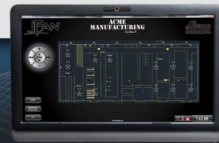
iFAN can be connected to facility's fire control system to command "All Stop" in the event an alarm is triggered.
