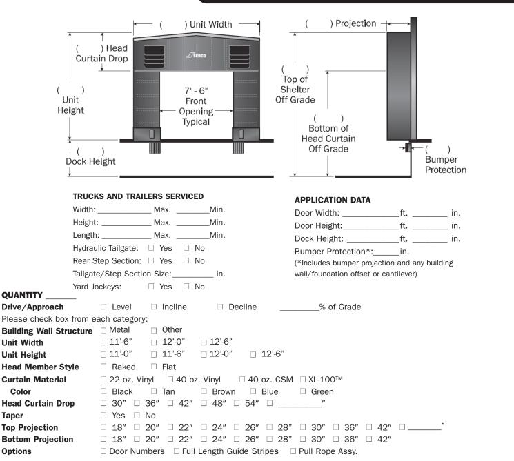
\*Note: Pressure Against Building Wall: S2200 exerts standard pressure against the building wall when a trailer is backed between the foam side frames. If the side frames are impacted by a backing trailer and compressed, higher building wall pressure can result. If the building wall pressure is of concern, steel protectors are recommended.
