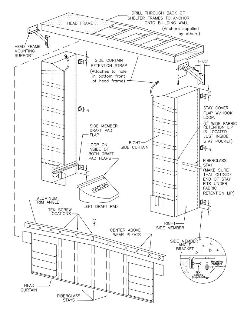
FOAM SIDE MEMBER MOUNTING DETAILS (MOUNTING ANCHORS NOT INCLUDED)
