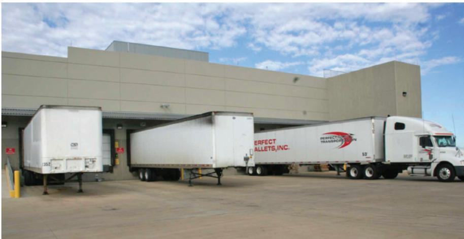
For years plant dock doors have been designed like garage doors. A forklift collision impact can take out a door panel, creating a gap between it and the doorframe.
