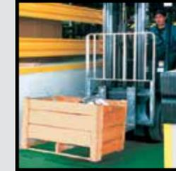
Unlike standard scissors lifts, the Kelley KD Series Kombo Dock's hydraulically powered dock lip ensures faster cycling times. With up to 20,000 lb. (9,072 kg) lifting capacity the Kombo Dock can handle the toughest loads while also providing dock-to-grade level forklift access.
