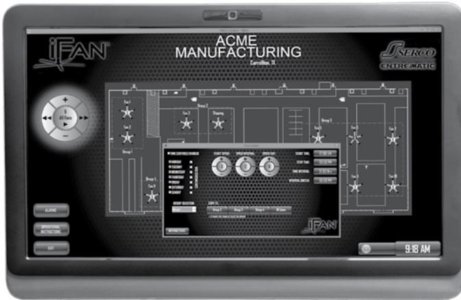
Timer setting dialog box enables direction and speed for individual HVLS fan or zones to be set by time of day.
